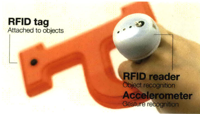
Figure 4 The OnObject device senses objects user grabs by an attached RFID tag and detects motion gestures the user makes with their hand.
