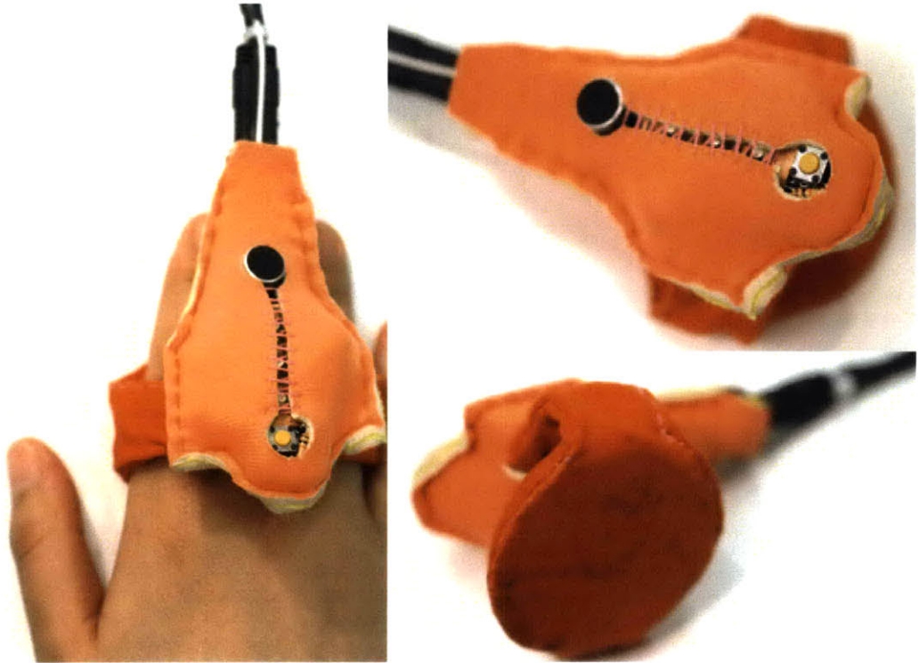
Figure 45 Soft device with elastic antenna band.
