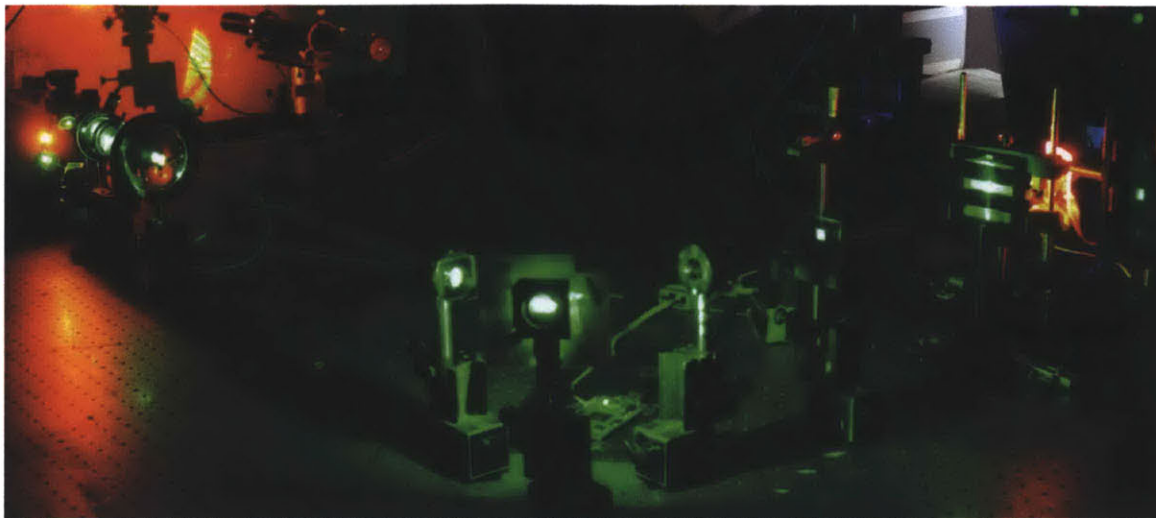
FIGURE 3.4: Photograph of the direct fringe writing setup. Left: DPSS laser, beam-expanding optics; center: LCoS SLM in cross-polarizer configuration; right: telecentric imaging optics and photorefractive polymer.
