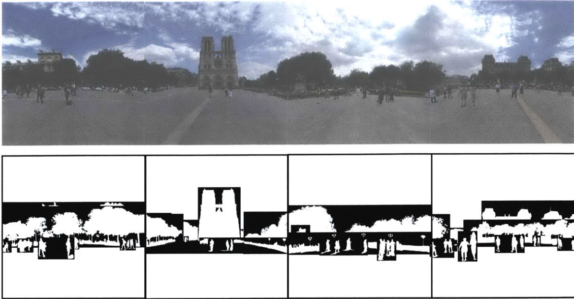
Figure 7-16: Panorama of Notre Dame, Paris (top). Alpha channels (bottom). The resolution of each image is 640 \times 640 . There are 43 layers total. The detailed segmentation process took about five hours. Specifying the depth took two hours.
