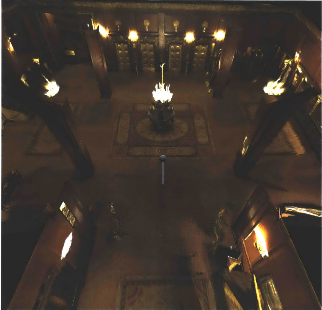
Figure 7-21: Bird's-eye view of the reconstructed hotel lobby. The grey sphere shows the acquisition position of the initial photographs. Note that parts of the scene further away from the acquisition position are pixelated and lose resolution, due to the sample-based representation.
