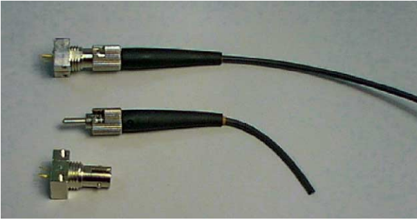
Fig. 8. Photograph of an ST fiber pigtail and the laser housed in an ST-connector is shown.
