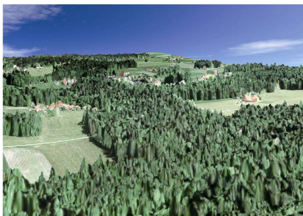
Fig. 3. Forest heights derived from the Pol-InSAR technique overlaid on a Google map from Traunstein, Germany (forest height retrieval based on two fully-polarimetric L-band data sets acquired by DLR's airborne E-SAR system).
