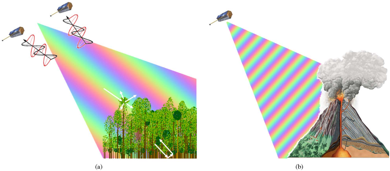
Fig. 16. Measurement modes of Tandem-L. (a) The 3-D structure mode employs polarimetric SAR interferometry to measure tree heights and vertical vegetation profiles. The individual contributions from ground and canopy are separated via their polarimetric signatures, and the corresponding heights are measured by cross-track interferometry. (b) The deformation mode employs repeat-pass interferometry to measure range changes with millimetric accuracy.
