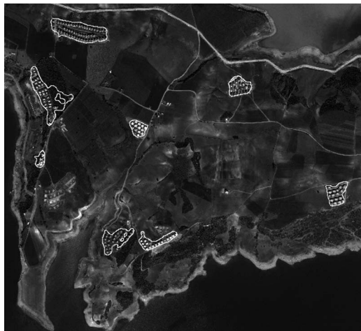
Fig. 1. Urban region detection results (detected boundaries labeled white) from the large Ikonos image acquired over Adana, Turkey.
