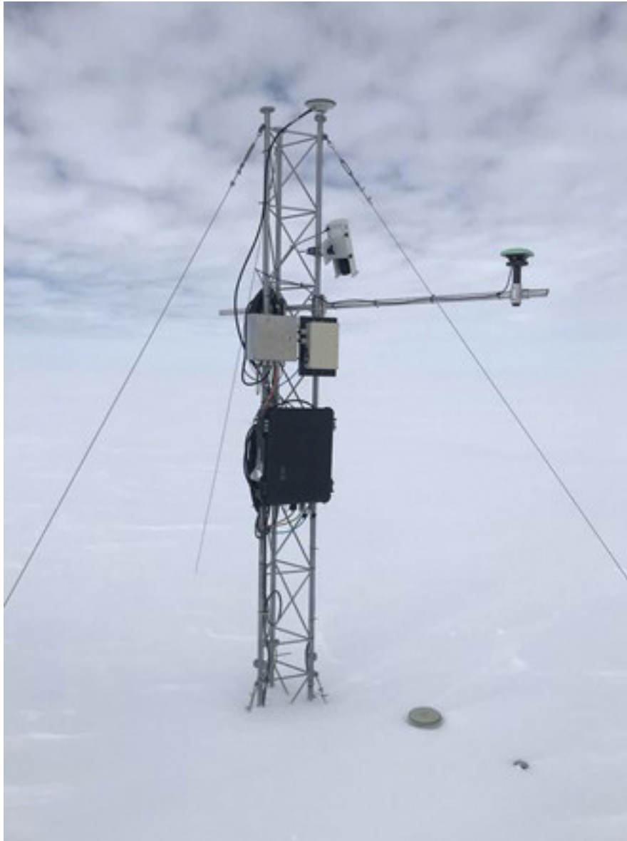
Fig. 4.19.1: GNSS snow monitoring system setup in the vicinity of the Neumayer Station III at the Ekström Ice Shelf on 22 November 2021, with view towards West; the GNSS antenna on top of the mast serves as a reference station and additionally collects reflected GNSS signals visible on the ground from the surrounding snow surfaces. The two lower GNSS antennas (one high-end and one low-cost) will collect refracted GNSS signals when fully covered and buried by accumulated snow. Power and LAN supply is provided by the nearby AWI air chemistry observatory (Spuso) and connected to the receivers in the black box.
