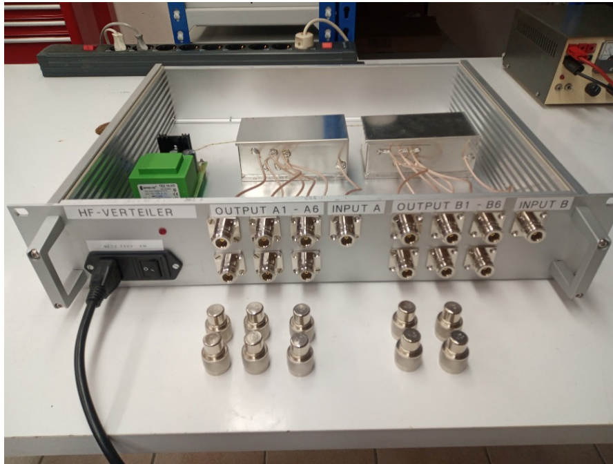
Fig. 4.10.1: New dual channel power preamplifier with 10 termination resistors in front of the open chassis
