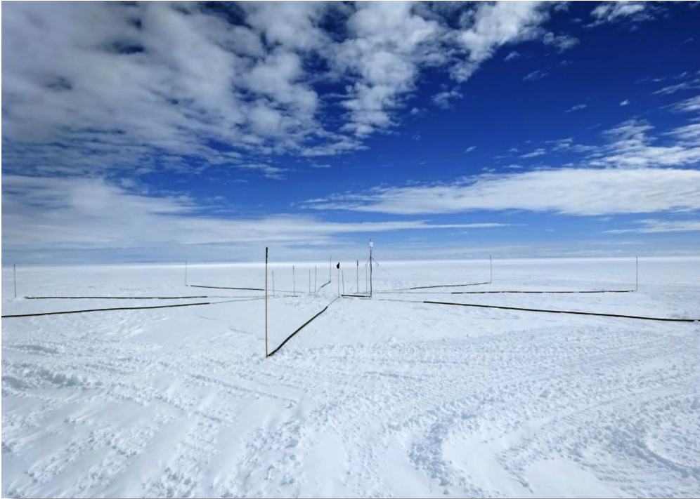
Fig. 4.4.2 One of the nine infrasound elements after recovering from snow. Flagpoles mark the outer positions of the air-pressure inlet-tubes which are part of the wind-noise-reduction-system. In the center, a field-box is buried in the snow. A WiFi-Link connects each element with the Neumayer Station III.
