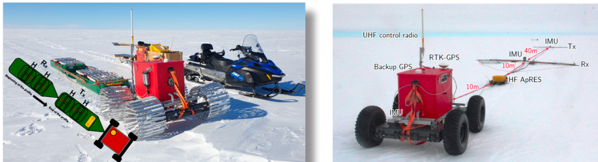
Fig. 4.18.3: Rover connected to the polarimetric VHF ApRES (left) and the HF ApRES (right).
