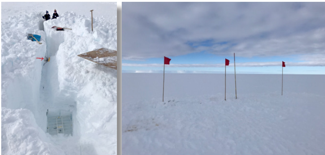
Fig. 4.16.2: Site MIMO-EIS-8: Retrieval of the ApRES system controller (photo left: yellow box in the center pit – indicated by red arrow) and two frame antennas (front and back pits) on 25 November and photo (right) of the site after completion of the new deployment on 26 November, with the system buried at about 20 cm depth below the current surface and system controller (two flags in center) and each frame antenna (left and right flag) covered with wooden boards. The Iridium antenna is mounted on the bamboo pole without flag.
