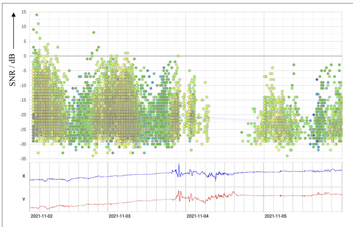
Fig. 4.10.4: The figure shows reported signal-to-noise-ratio of the transmitter spots during the event on 2 November and the magnetic components x and y .
