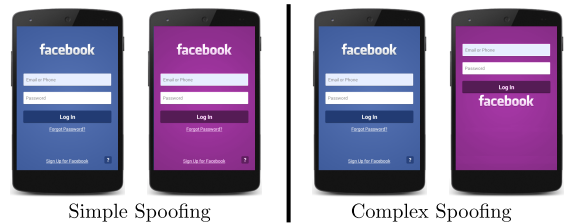
Figure 2: Examples of simple (changing background color) and more complex spoofing (repositioning elements).
