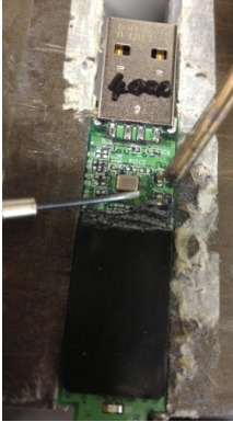
Fig. 4: Epoxy removal of Kingston DT 5000 with screwdriver
