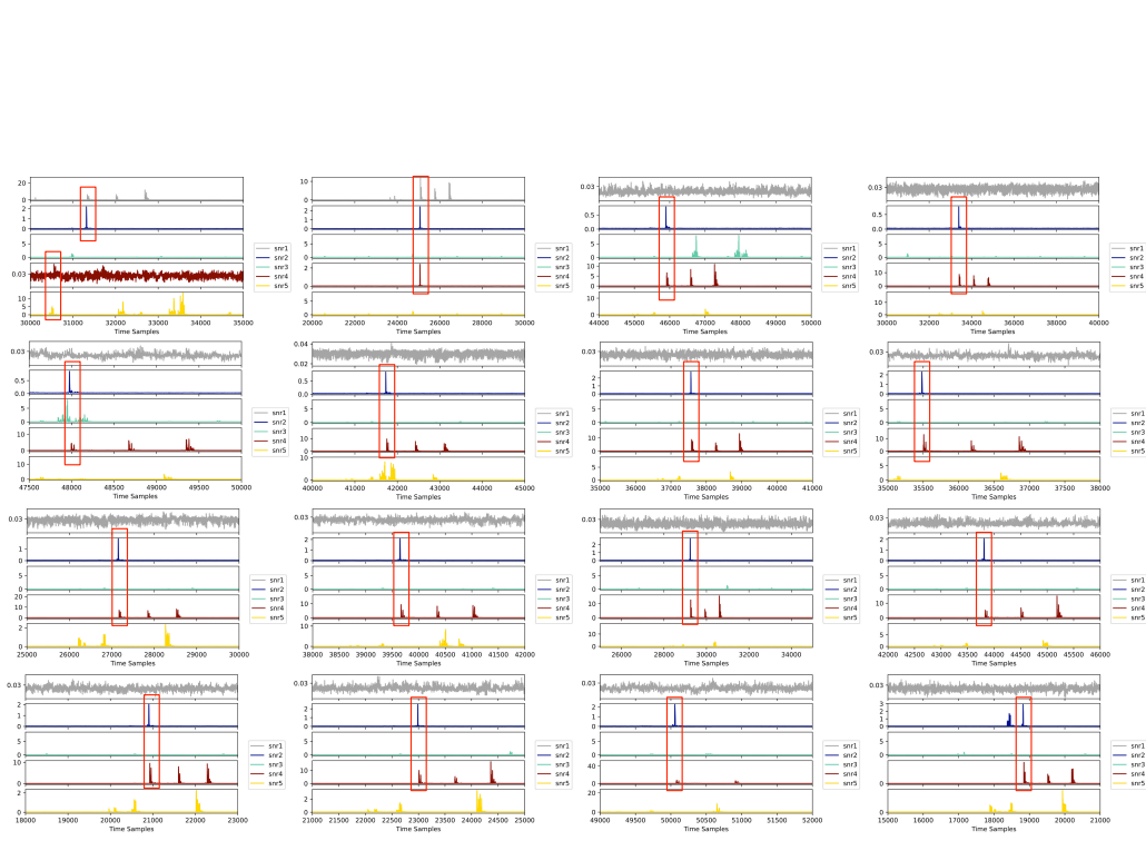
Figure 11: Detailed SNR of 16 S-boxes
