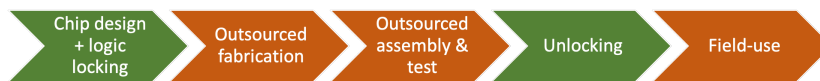
Figure 2: IC supply chain in the presence of logic locking that protects against the untrusted foundry, test facility, and end user. Note that after chip fabrication and testing, the chip is unlocked by loading the correct key onto the memory of the chip.
