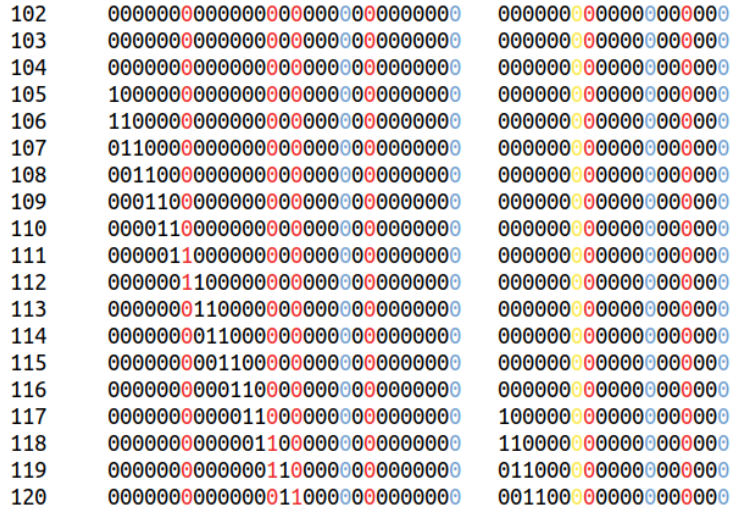
Fig 5: Experimental demonstration of a MAND occurrence. The figure shows the last few rounds trail of the 60-round (120 iterations) KATAN48 related-key distinguisher. In the figure, left, middle and right columns refer to the iteration number, bit-differences in L_2 and L_1 register respectively. In the L_2 register, the red-colored bits denote the position 6, 13, 15 and 21 (starting from left).
