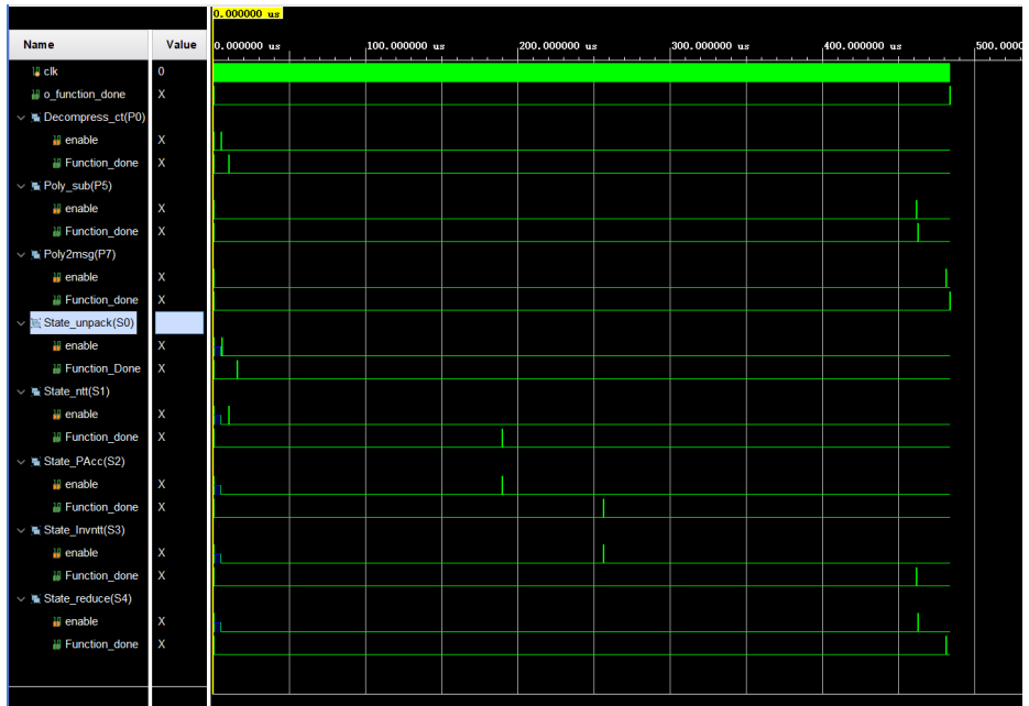
Fig. 9: A timing simulation using Xilinx Vivado Design Suite. The module called Poly2msg(P7) corresponds to State.Polytomsg() .
