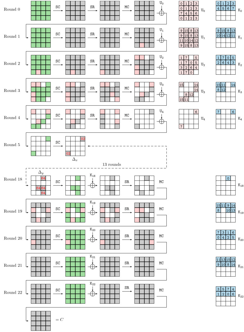
Figure 3: 23-round attack on SKINNY-128-384 [BDD + 23]. The blue key bytes are needed to compute the values of green ones. Both white and red bytes have zero difference, but the red ones are required to compute green bytes.
