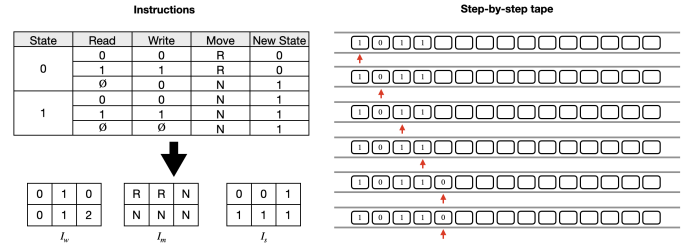
Figure 1. An illustration of a classic Turing Machine (TM) designed to perform binary multiplication by 2 (with the alphabet being \mathbb{B} and the blank symbol). The red arrow represents the head of the TM. The machine's instructions are documented in a table that can be expressed as three matrices: I_w for writing instructions, I_m for moving instructions, and I_s for state-changing instructions. The behavior of the TM will depend on the cell content under its head and the current state.
