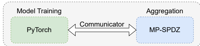
Figure 1: High level overview of SAFEFL framework, comprising of the Model Training module using PyTorch [75] and the Aggregation module using MP-SPDZ [47] along with the communicator interface between them.
