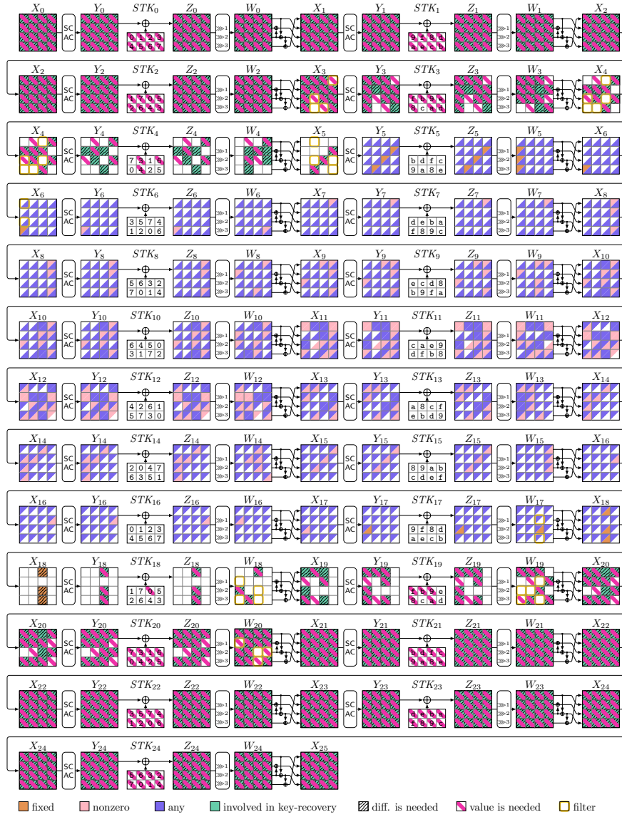
Fig. 13: ID attack on 25-round SKINNYe-v2. c_b = 16c, c_f = 16c, r_b = 16c, r_f = 16c, |k_b \cup k_f| = 63c, |k_b| = 34c, |k_f| = 46c
