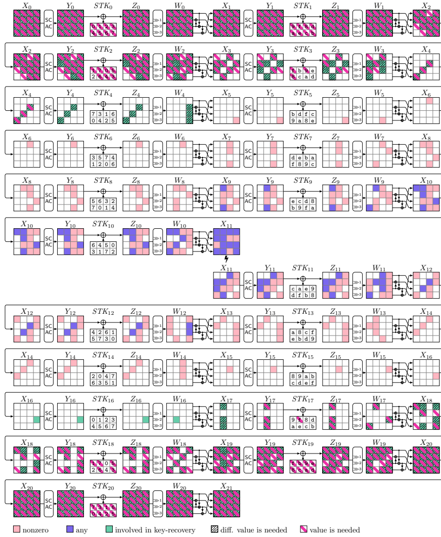
Fig. 7: ID attack on 21-round SKINNY- n-3n . c_b = 15c, c_f = 15c, r_b = 16c, r_f = 16c, |k_b \cup k_f| = 42c, |k_b| = 26c, |k_f| = 22c
