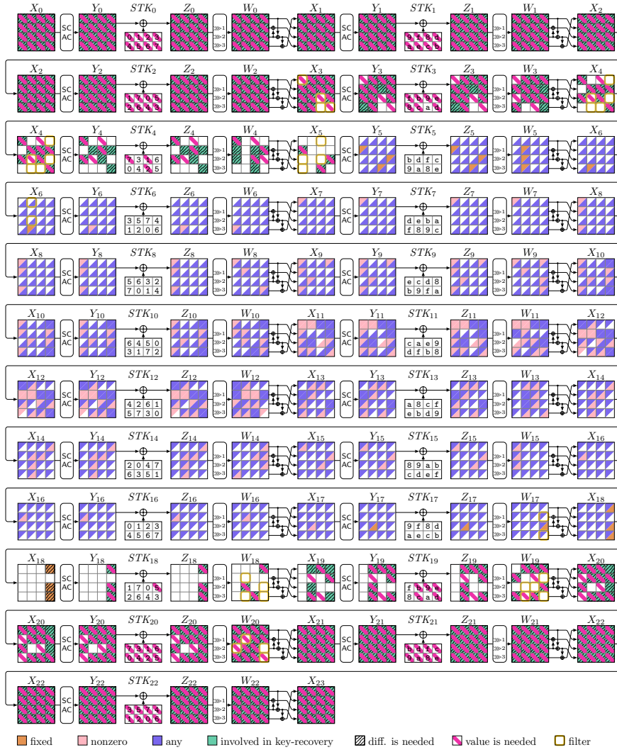
Fig. 11: ID attack on 23-round SKINNYe-v2. c_b = 16c, c_f = 16c, r_b = 16c, r_f = 16c, |k_b \cup k_f| = 60c, |k_b| = 34c, |k_f| = 30c
