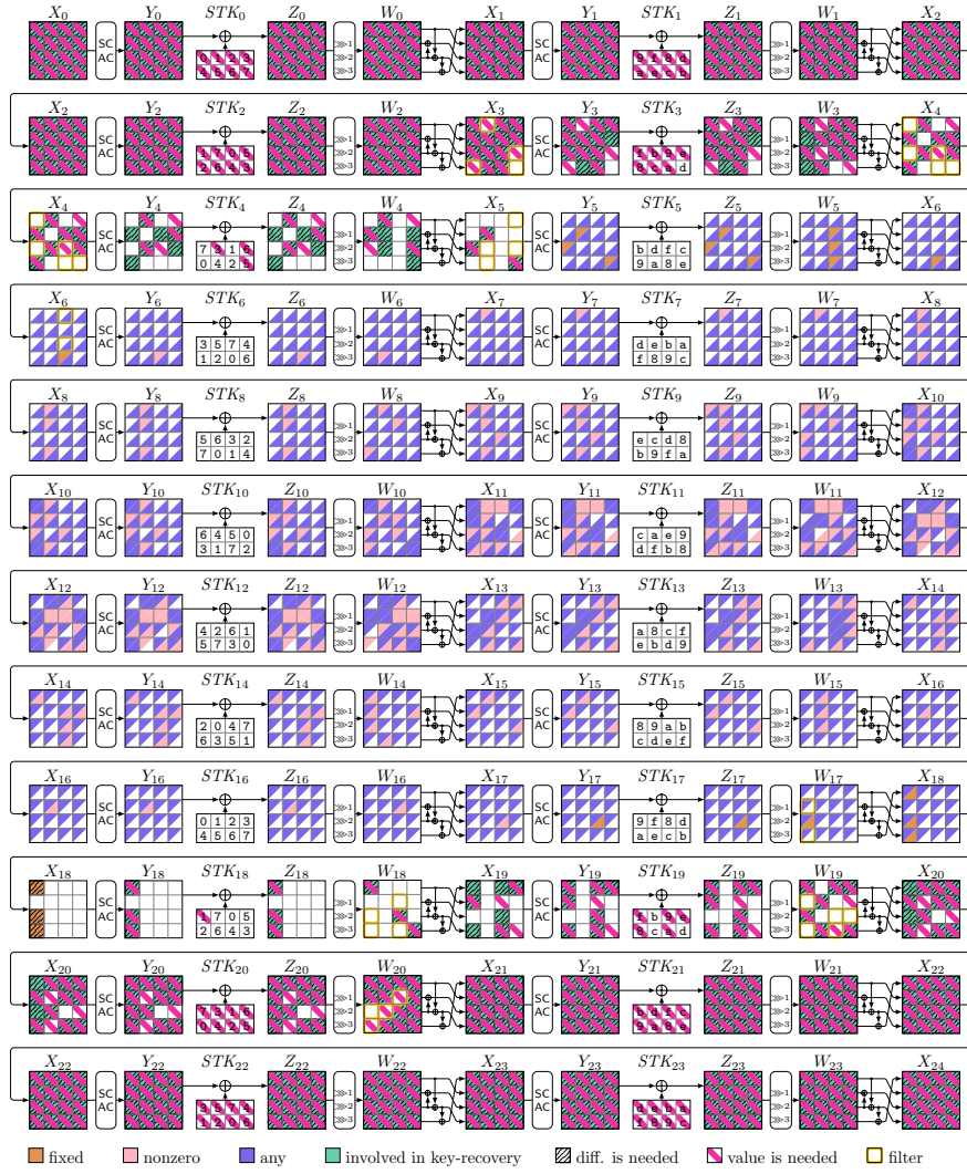
Fig. 12: ID attack on 24-round SKINNYe-v2. c_b = 16c, c_f = 16c, r_b = 16c, r_f = 16c, |k_b \cup k_f| = 63c, |k_b| = 34c, |k_f| = 38c
