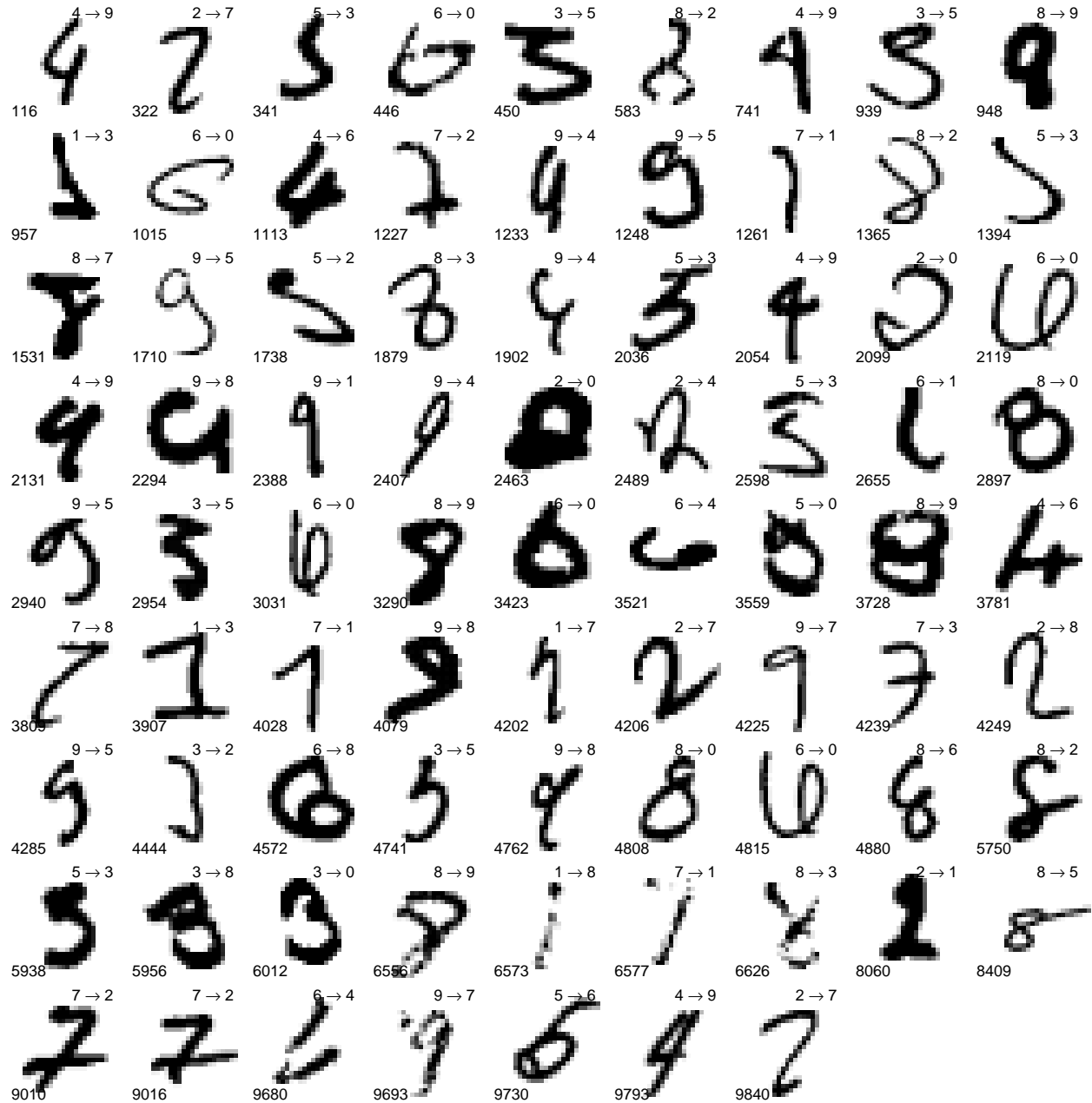
Figure 2.6: All the errors made by the classifier on the MNIST dataset. On each image a \rightarrow b means that the digit a was misclassified as b .
