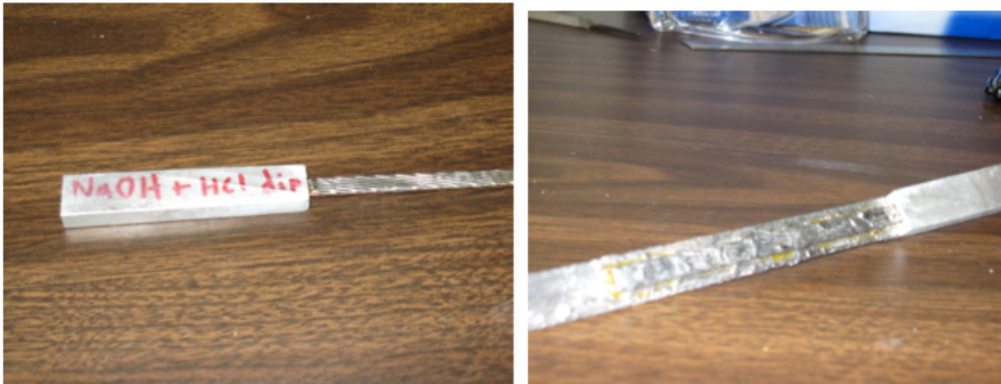
Figure 7.63 a) Chemical Etching of Aluminum Stabilized NbTi Conductor. b) Successful Solder Joint.
