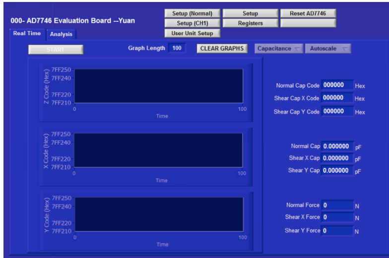
Figure 43 Screenshot for LabVIEW program user interface for testing AD7746
