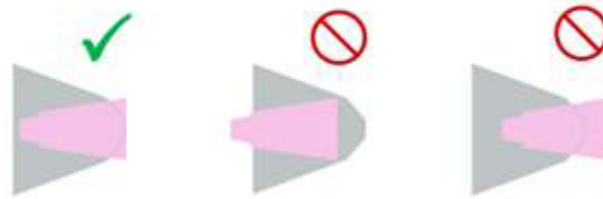
Figure 66: Proper placement of cannula relative to head of mouse. Diagram courtesy of Zineb Idrissi and Dr. Annette Roubichaud of SCIREQ.
