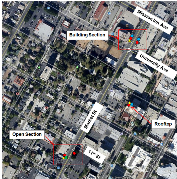
Figure 5.6 Location of instruments in May 2015 Riverside, CA, field study. ●—Condensation Particle Counter (CPC). ●—AQMesh. ▲—Sonic Anemometer. ■—Camera. Map Data: Google.
