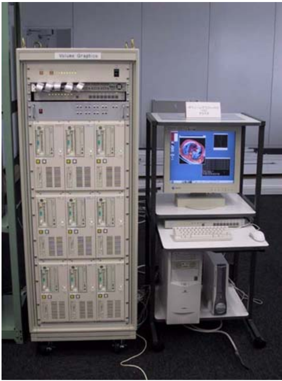
Figure 9: The prototype of the visual computing cluster.
