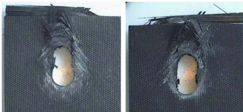
Fig. 26: Laminates after bearing failure of bolted joints [97].
