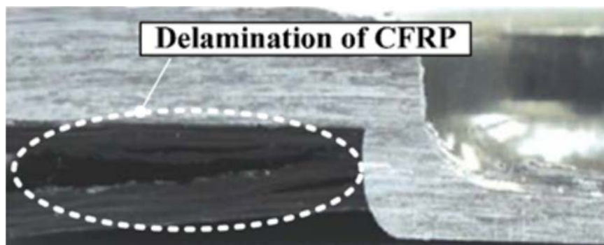
Fig. 35: Delamination of CFRP laminates in hole-clinched joints [117].
