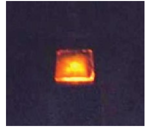
Left: At layer of silver was coated on fluorescent material. Light emission efficiency is low due to energy lose in total internal reflection.
