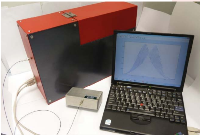
Wide dynamic range phase-sensitive surface plasmon resonance sensor 寬動態範圍相位敏感表面等離子體共振傳感器
