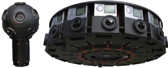
360-degree cameras 360度攝像設備
