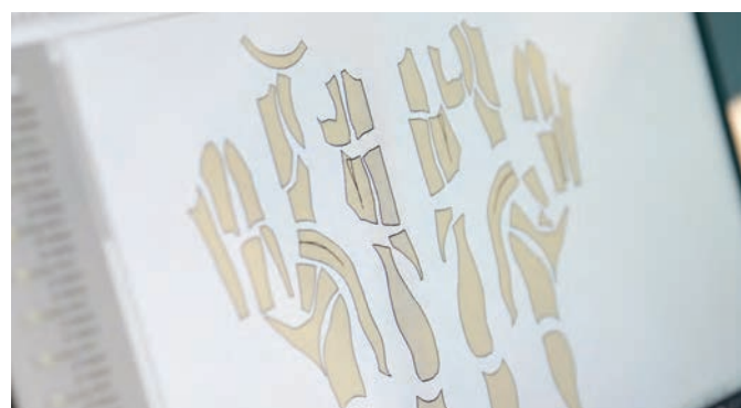
2D flattened layout for final cutting and wiring 二維紙樣作剪裁及縫接
