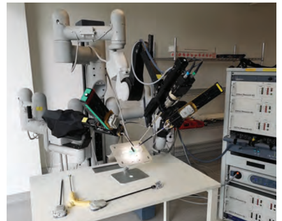
OCTRVS integration with da Vinci surgical robot OCTRVS與達芬奇手術機器人
