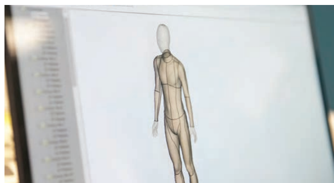
3D human model with pre-designed wetsuit layout 三維人體模型上套用了預先設計的潛水服
