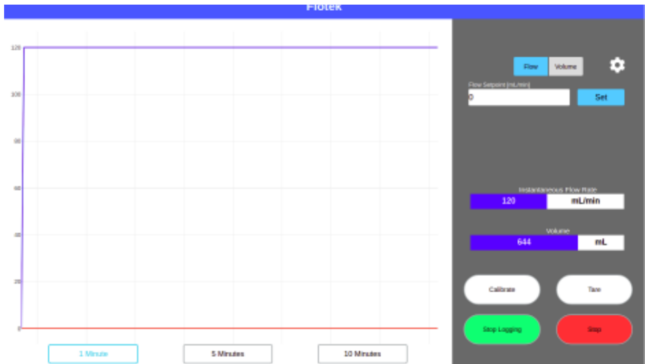
Figure 3: Controller In Logging Mode. Note the “Stop Logging” State of the logging button and the green color
