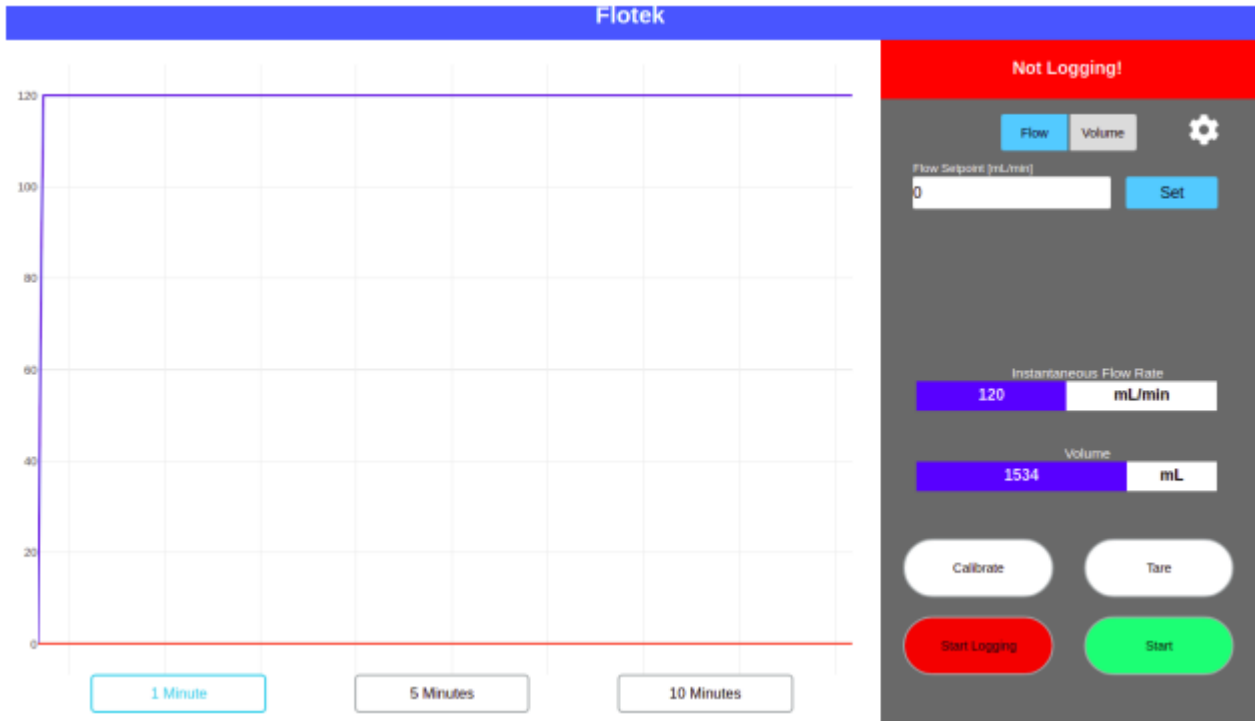
Figure 7: Shortly after pressing the Stop button. Note the Color and State of the Start/Stop Button This is the state present at boot
