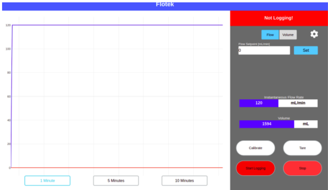
Figure 8: Controller In Running mode with user prompt to stop graphing.
