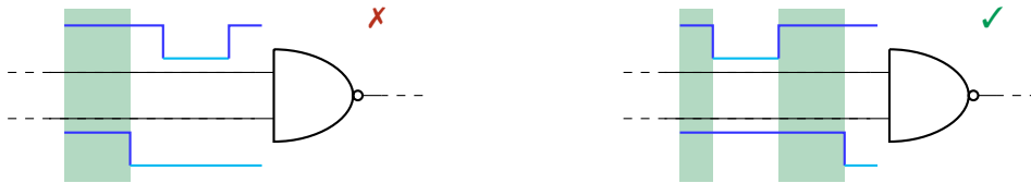
(a) The glitch occurs after the initialization and (b) The glitch occurs before the last initialization and the test is valid.
