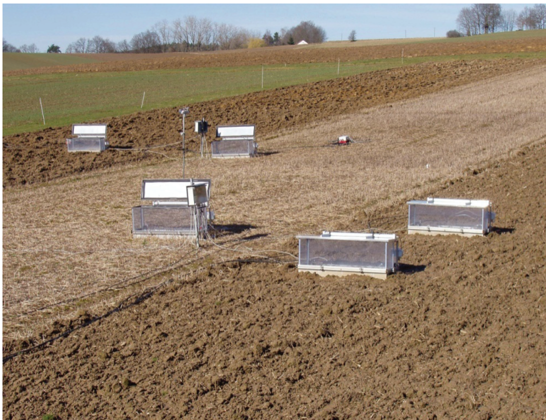
Fig. 16. Trace gas flux observation with automated chambers on field plots at the TERENO station Scheyern.
