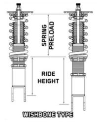
NEVER over extend strut assembly. These are lowering kit that at max length will still be at least 30 MM lowered from factory ride height.
