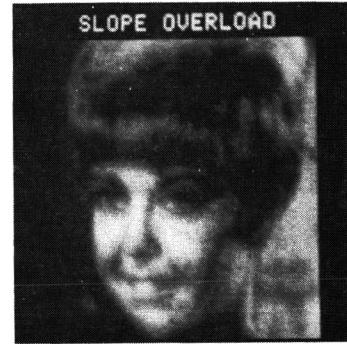
FIGURE 3B, 3 LEVEL DPCM CODING OF KODAK GIRL. THE CHOSEN LEVELS ILLUSTRATE SLOPE OVERLOAD
