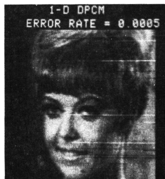
FIGURE 3D, 1-D DPCM CODING IN THE PRESENCE OF 0.0005 BIT ERROR RATE.
