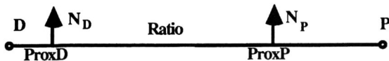
Fig.9. Normal interpolation for a tampon area. N_P = original normal for the proximal joint, N_D = original normal for the distal joint; the interpolated normal is computed as: R' N_D + (1-R') N_P with R' = Ratio - \frac{ProxP}{1-ProxD} - ProxP
