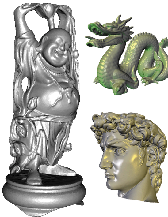
Figure 1: Scanned meshes from Stanford 3D model repository [26]. All three meshes are valid 2-manifolds: the Buddha has genus 104, the dragon has genus 46, and David's head has genus 340. Most of these tunnels/handles are noise and can be safely removed.
