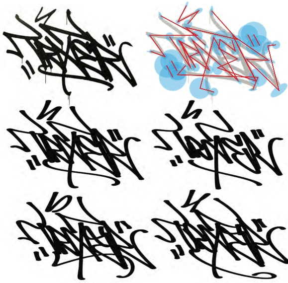
Figure 10: Top left, a graffiti script (tag) made with a marker by Los Angeles artist “Trixter”. Top right, a user defined “motor plan” for the tag, generated by placing targets near salient positions along the original trace and then adjusting the covariances to follow the original trajectory. Second row, the reconstructed trajectory (left) and one variation made by increasing the regularisation parameter r . Bottom row, two random samples from the corresponding trajectory distribution.
