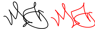
Figure 9: Automatic ligature generation by concatenating the control points of two letters. On the right, a comparative example using Bézier curves.
