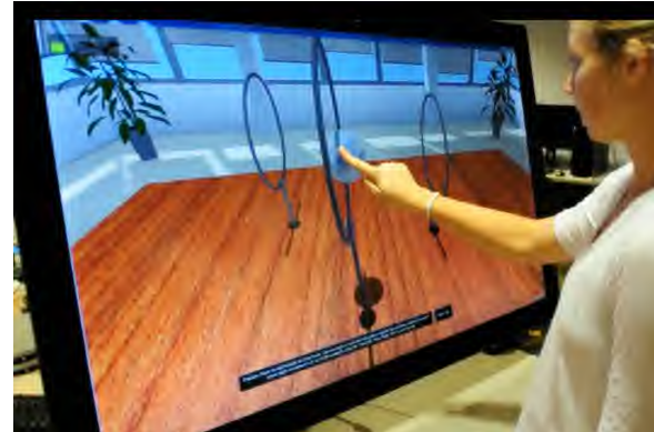
Figure 1: Our experiment apparatus included a 55-inch Perceptive Pixel display raised to standing height and tilted upwards by 30 degrees.
