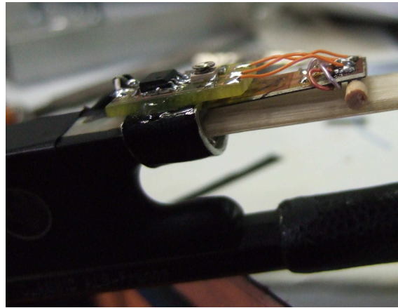
Figure 7. Bow force sensor. A thin steel strip is clamped to the flat side of the ferrule. The strip bends as the deflected bow hair presses at the free end via a wooden bearing piece. The bending is measured by two strain gauges glued to the strip. A Wheatstone bridge and conditioning amplifier is integrated in the sensor.
