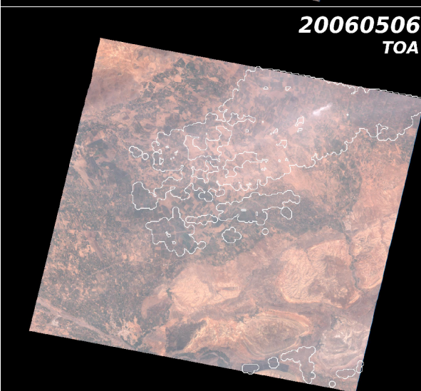
Figure 5 : visual verifications for a few cases identified in figure 3. White lines correspond to cloud contours from MTCD method. Upper Left) MTCD gives 12% of cloud cover, NSPO: 0%. Very small clouds can be seen, that were not seen by the operator. Upper Right) MTCD 80%, NSPO: 20%. Here, the operator probably only considered the thick clouds at the bottom of the image, but most of the image is evidently covered by thin clouds. Middle left) MTCD : 34%, NSPO 55%. The image is covered by small clouds, all of them seem to have been detected by MTCD. The operator has probably considered part of the space between clouds as cloudy. Middle right) MTCD 37%, NSPO 85%, the thin cloud cover is underestimated by our cloud mask because the previous image in the time series is quite old. Bottom Left) MTCD 22%, NSPO 0%. Thin clouds were not classified as clouds by NSPO operator. Bottom Right) MTCD 42%, NSPO 20%. The MTCD cloud cover looks accurate.
