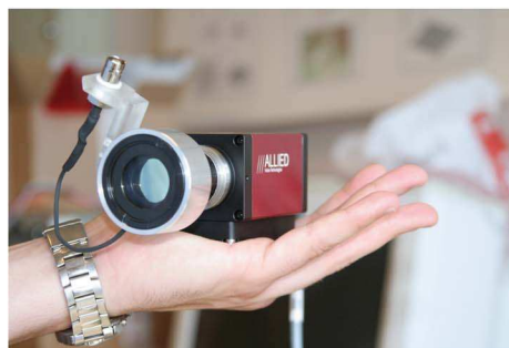
Fig. 1. (Color online) Polarimeter scheme and photo. The modulator is composed of an FLC cell and a linear polarizer.
