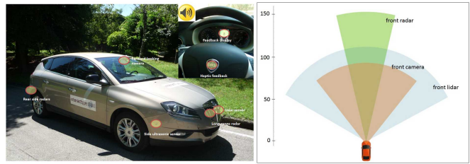
Figure 3. Left: images of the CRF vehicle demonstrator. Right: Field of view of the three frontal sensors used as inputs to gather datasets for our proposed fusion approach detailed in Sections VI, VII and VIII.
