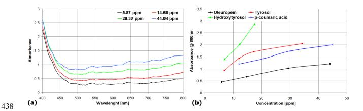
**Fig. 2**. Measured absorbance vs. wavelength in the range 400 - 800 nm for different concentrations of oleuropein (a) and measured absorbance at 800 nm plotted vs. phenol content for different phenolic compounds (b).
