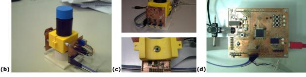
**Fig. 5**. Schematic of the electronic board of the embedded system realized in the present work (a); pictures of the sensor (b) and (c); photograph of the electronic board (d).
