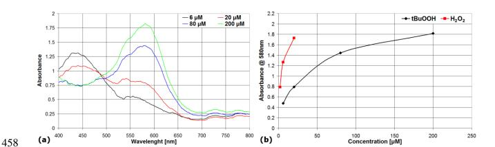
**Fig. 3**. Absorbance plotted vs. wavelength in the range 400 - 800 nm for different concentrations of tert-butyl hydroperoxide (a) and measured absorbance at 580 nm plotted vs. concentration for tert-butyl hydroperoxide as well as vs. hydrogen peroxide (b).
