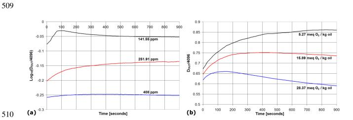
**Fig. 6**. Data measured with the designed electronic board for different oil samples vs. time in the case of total phenol content (a) and peroxide value (b).
