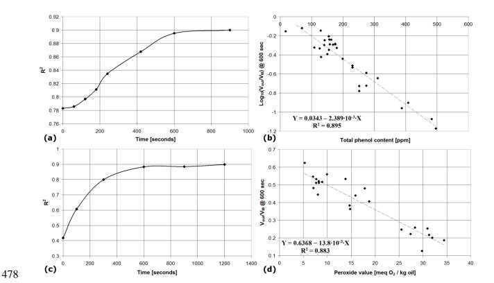
**Fig. 4**. Coefficient of determination  $R^2$  plotted vs. time for the total phenol content (a) and peroxide value (c). Scatter plot and linear regression line calculated for 600 seconds for total phenol content (b) and peroxide value (d).
