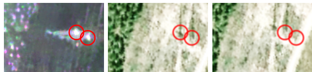
Figure 26. Example of a common pylon selection: on the polarimetric SAR image on the left, on the optical image coregistered by GeFolki in the middle, and coregistered by geocoding on the right. Red circles indicate the position of the pylon bases in the SAR master image.
