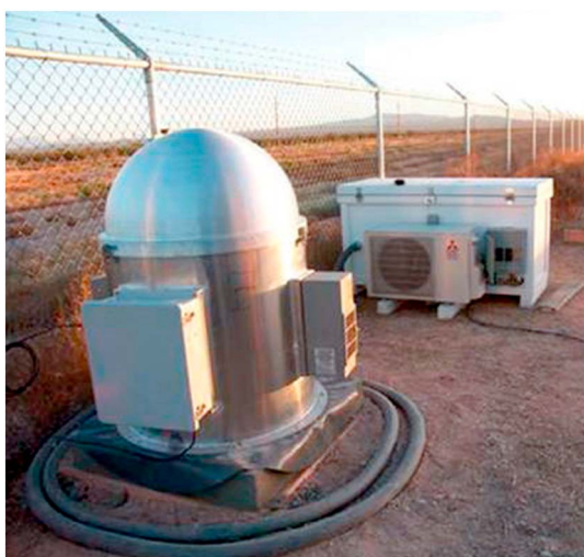
Figure A6. iGrav superconducting gravimeter inside its field enclosure. Credit: GWR Instruments, Inc.
