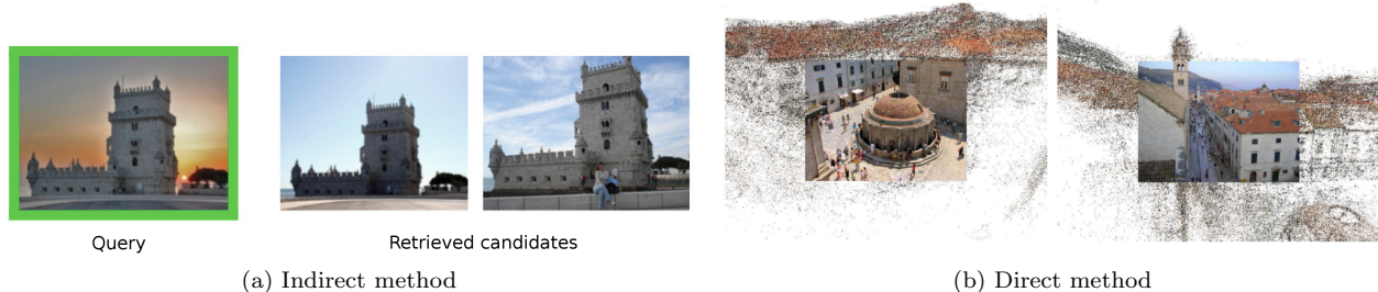
Figure 1: Examples of Visual Based Localization systems: (a) indirect method from [160]: according to an input query (left images), indirect methods recover a set of similar data (right images). (b) direct method from [49]: direct methods recover the exact pose of the input query (the two figures represents superposed images according to a reference 3D model).
