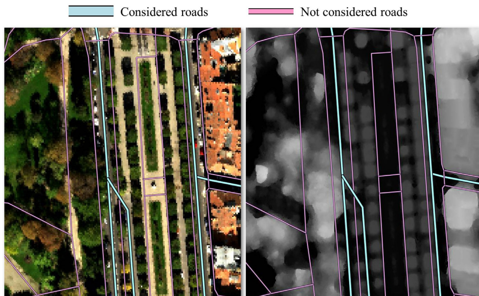
Fig. 3. Illustration of the data used in this study for the first site. Left: VNIR reflectance image. Right: DSM. The GIS data is represented by blue and violet lines indicated over the airborne data. (For interpretation of the references to color in this figure legend, the reader is referred to the web version of this article.)
