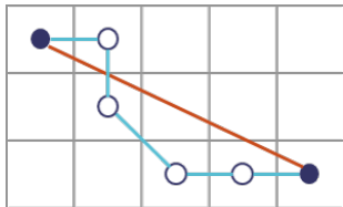
Fig. 1: Interest of spaced out waypoints. The waypoints, centered in square cells, are represented by circles.
