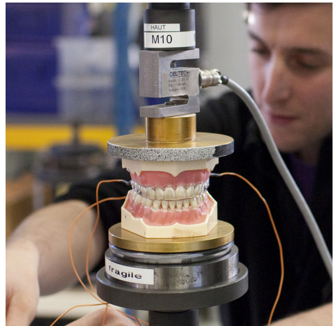
Figure 8. Overview of the experiment for in vitro characterization of the sensing system
