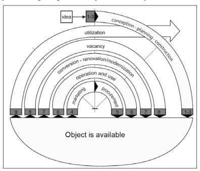
Figure 1. Life cycle phases in FM (GEFMA 100-1, 2004).
