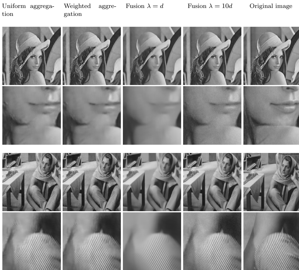
Fig. 11: Comparison of the different aggregation procedures on Lena and Barbara , using HDMI for the inference of Gaussian models. Images are degraded by a noise of standard deviation \sigma = 30 .
